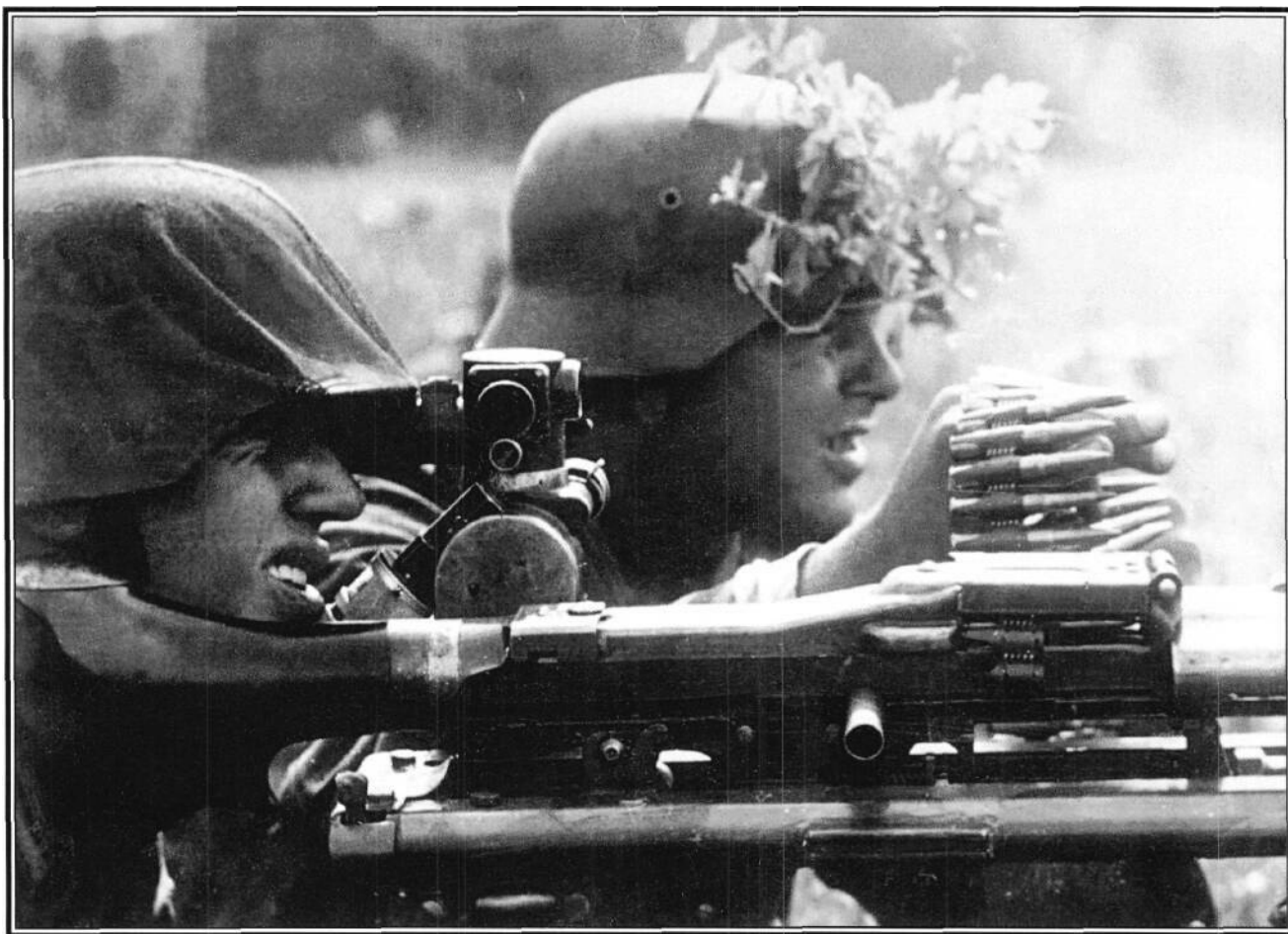
Above: While Soviet troops prepare to attack, German troops nervously await them. These soldiers man an MG 34 machine gun on a sustained-fire mount, capable of firing 800–900 rounds per minute.
