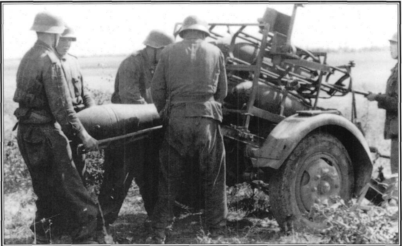
Above: 300mm (11.9in) rockets are loaded onto a Nebelwerfer ready to fire on Soviet positions in support of Model's troops. The trailer could be towed behind a light vehicle, making it fast moving.
